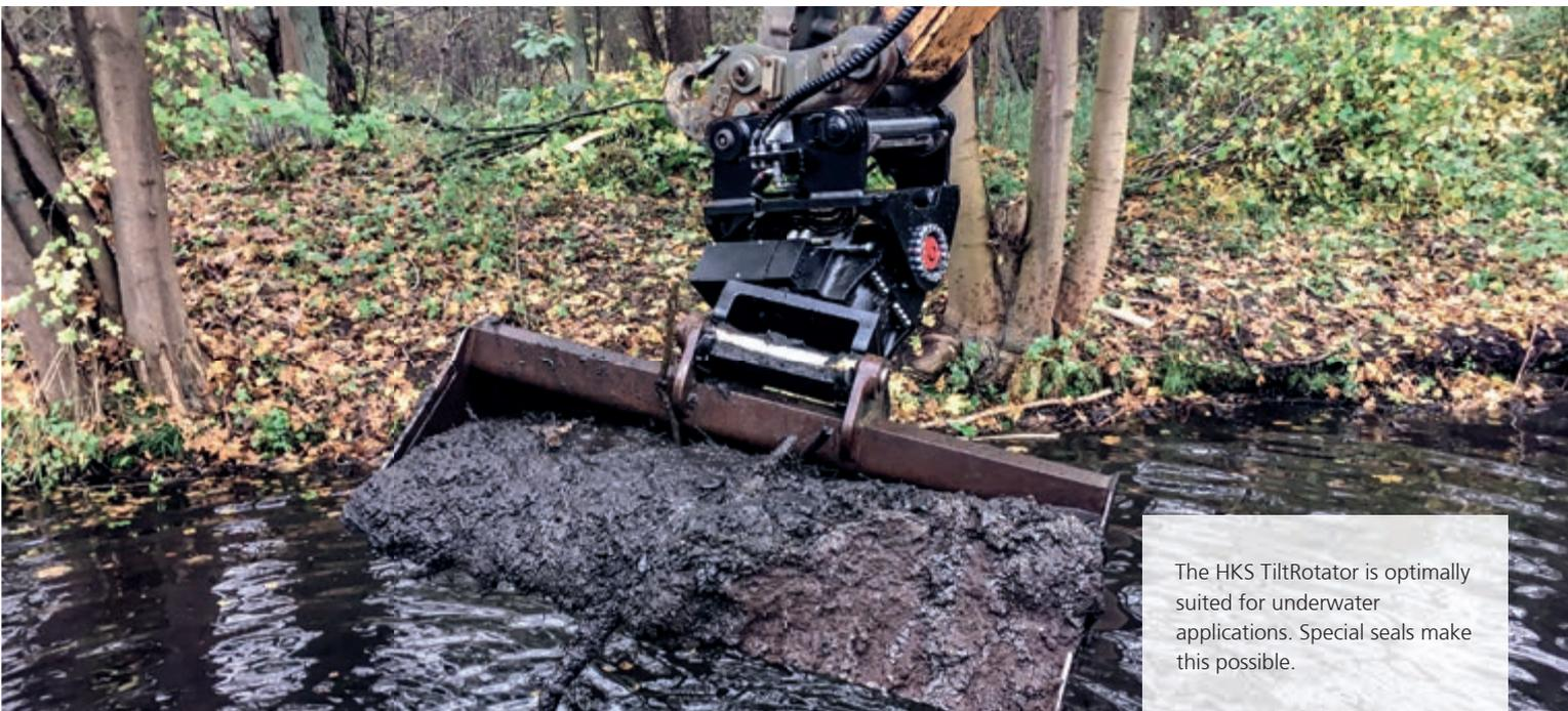
The HKS TiltRotator is optimally suited for underwater applications. Special seals make this possible.
